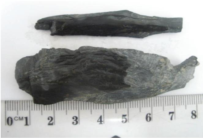
Figure 5. Splintered shale cuttings from 2170 mMD in Ungani-1.
