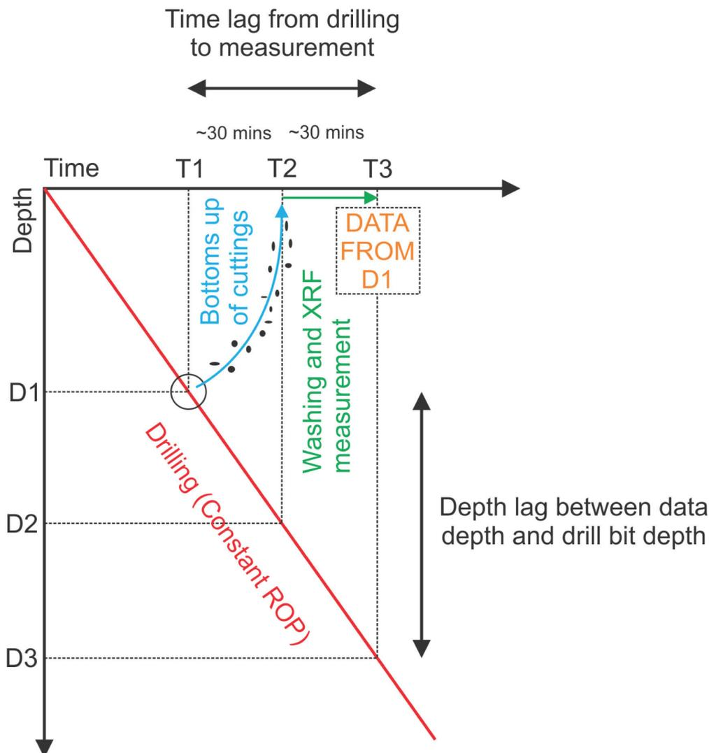
**Figure 9.** Wellsite analysis timings, demonstrating lag time and sample processing time while drilling.
