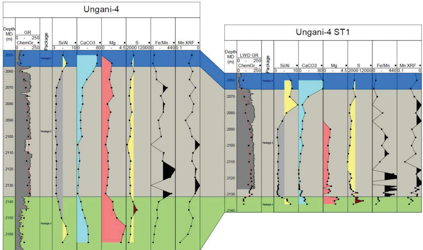
**Figure 7.** Ungani-4 ST1 wellsite XRF analysis data with Ungani-4 for comparison. High Si/Al in the Ungani Dolomite (Package 4) indicates the quartz-rich nature of the siliciclastic material present in this well.
